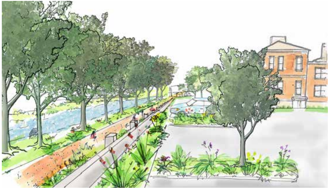
Parking lots in town could have bioretention basins to capture stormwater and pollutant runoff, and provide valuable pollinator habitat.
